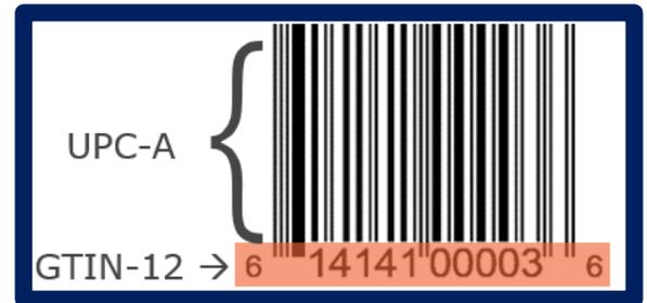
It is also important to draw a distinction between the barcode, in this case the UPC-A, and the data encoded, which in a UPC-A is always a GTIN-12. The GTIN-12 is one of four GTIN data structures. Internationally, the most commonly used GTIN is the GTIN-13, which is encoded in EAN-13 barcodes. EAN-13 barcodes are another member of the EAN/UPC family. For more guidance on GTINs, see the [GTIN Management Standard](#) and the [10 steps to barcode your product](#) guide.
