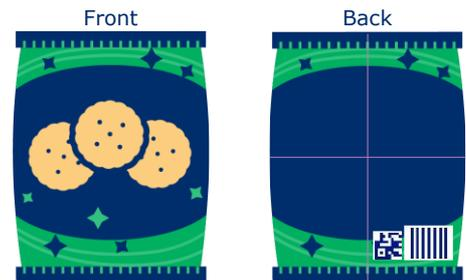
Adjacent placement also allows for a transition from an EAN-13 or UPC-A to dual marking to a sole 2D barcode while maintaining consistent symbol placement. When placing adjacent symbols, each symbol's quiet zones and other symbol placement rules must be respected. The orientation (stack or a row of symbols) or sequence (which symbol is placed on the left, right, top, or bottom) is determined by the brand owner.
