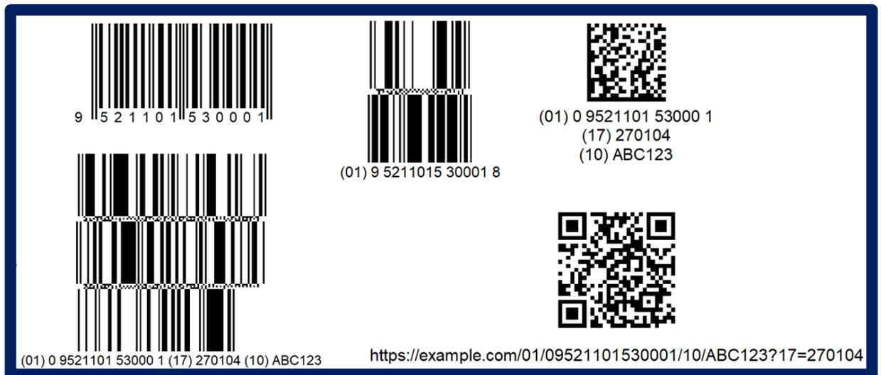
Above are examples of an EAN-13 and GS1 DataBar Omnidirectional Stacked barcode, encoding just a GTIN. A GS1 DataMatrix, GS1 DataBar Expanded Stacked encoding GS1 element string syntax and a QR Code encoding GS1 Digital Link URI syntax encoding GTIN, expiration date and batch/lot number. All examples use target sizing.
