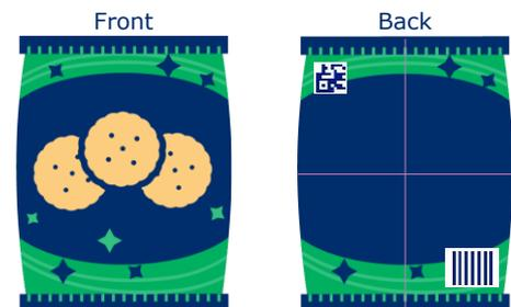
The guidance for hang tags is generally the same as for product packaging. Place the EAN/UPC in the same location as always and the 2D barcode on the other side of the tag, or in a different zone on the tag.
